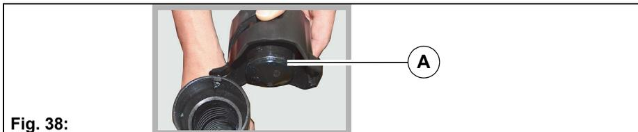
1. Twist drain valve by 90° and swivel down from drain hose.
